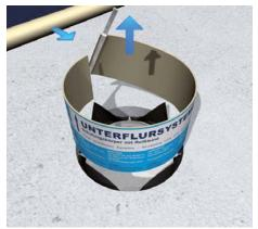
**6** | **Removal of shuttering pipe** Remove shuttering pipe with the release cord from the hardened screed. Process floor cover to the cleaned assembly opening (Ø 260 mm, Ø 308 mm).
